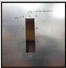
Countersink the top and bottom centre holes and cut out the centre slot.
