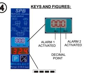
Note: The display remains switched off after 5 minutes of normal operation. Pressing any key the display value is visualised again.
