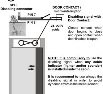
The SPB must continuously receive a blocking signal during all the time the lift is travelling, from the moment the doors are closing until the cabin gets on floor and the lift opens doors again. NOTE: Continuously. (Voltage 24-220Vac/dc)
