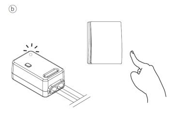
While the indicator on receiver flashes, press the Kinetic switch ONCE to complete the pairing.
